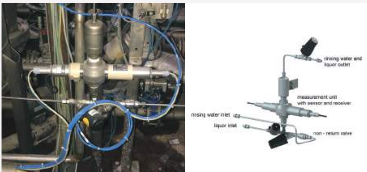
Figure 6.4: Thies DyeControl installed in an existing iMaster H 2 O exhaust dyeing machinery at a textile finishing plant in Lahore. © Thies
